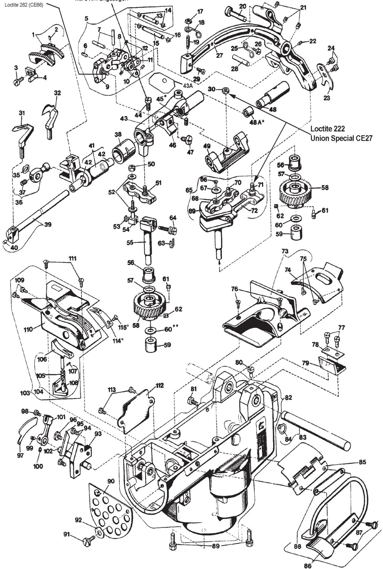
HOUSING, CRANKSHAFT, NEEDLE-, LOOPER-, FEED- AND CHAINCUTTER MECHANISM, FEED DOG, LOOPER, THROAT PLATE, COVERS
