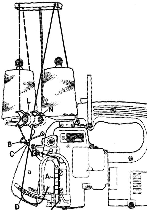
Diagram for two thread double locked stitch, type 401.
