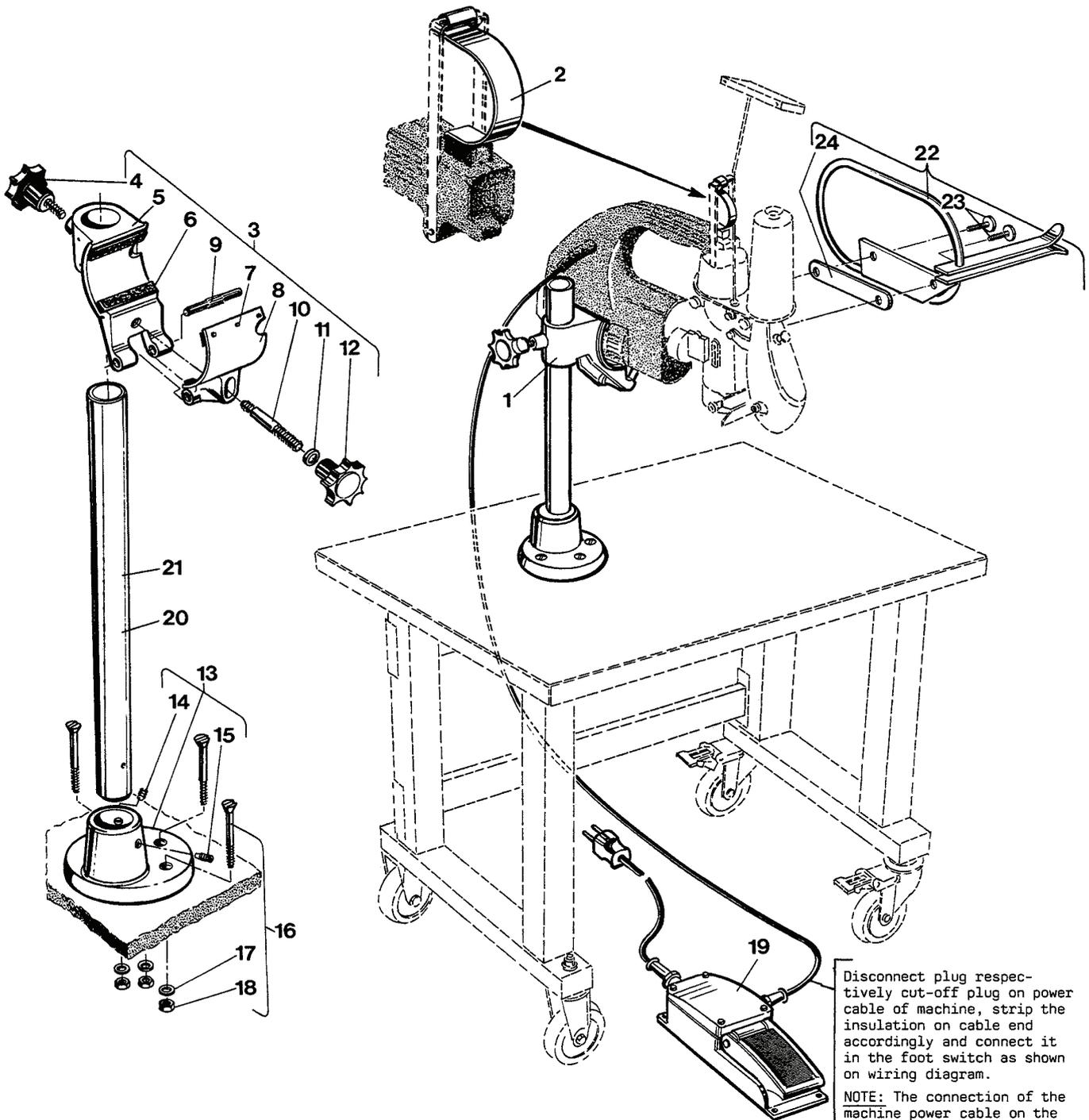
Disconnect plug respectively cut-off plug on power cable of machine, strip the insulation on cable end accordingly and connect it in the foot switch as shown on wiring diagram.
