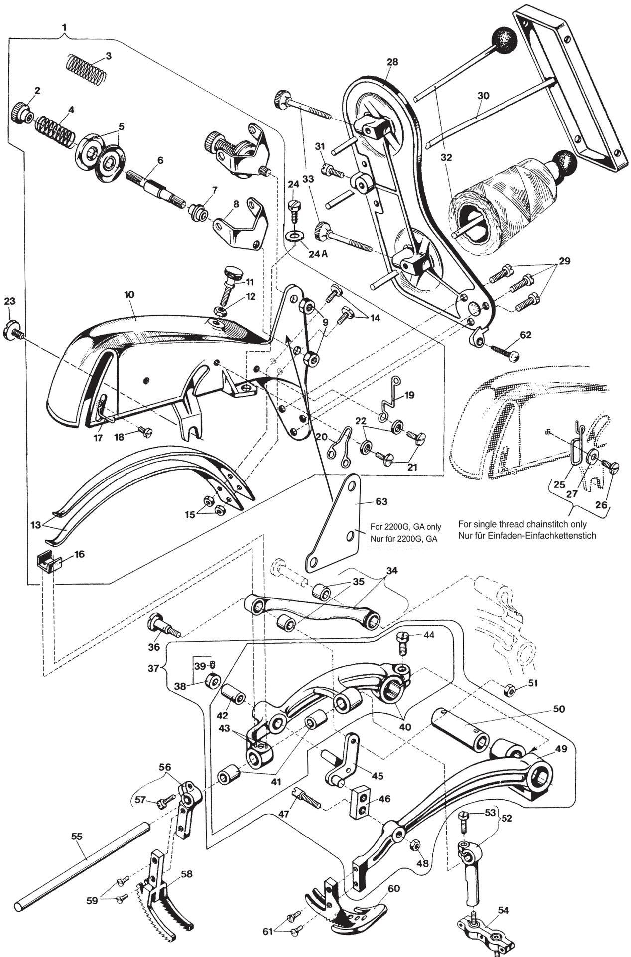
COVER ASSEMBLY, THREAD CONE SUPPORT, UPPER FEED DRIVE MECHANISM, PRESSER FOOT LEVER, UPPER FEED DOG, PRESSEER FOOT, THREAD GUIDES
