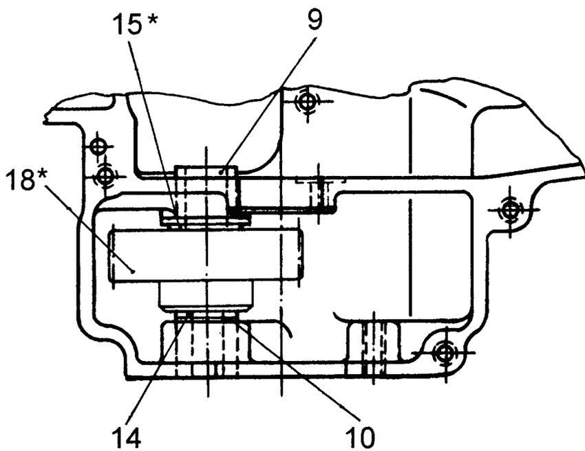
HOUSING ASSEMBLY, BUSHINGS FOR LOOPER SHAFT
