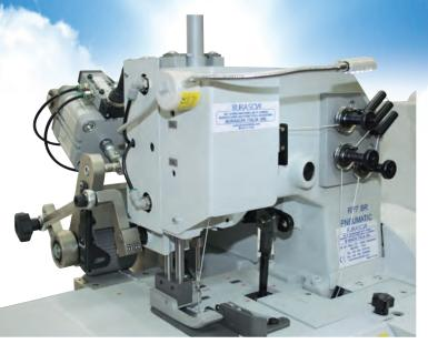
Detail of the net sewing machine RP7 BR PNEUMATIC, showing the operational area and many key components made from solid of the AISI 315 special alloy.
