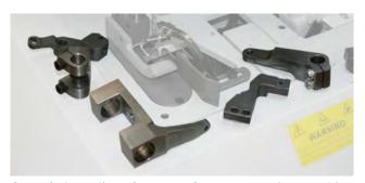
One of the salient features of our net sewing machine BURASCHI RP7 BR PNEUMATIC is that the key components are specially made from solid of the AISI 315 special alloy, extremely superior to the casted components of the traditional machines. In addition, our key components, heat treated with differentiated application in the critical area, are extremely strong, durable and reliable.
