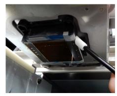
(4) Wipe the resin part between the print head's nozzle surface and nozzle guard.
