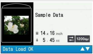
The print data loading will be completed when the print button stops blinking and remains lit, while the electric chime sounds.
